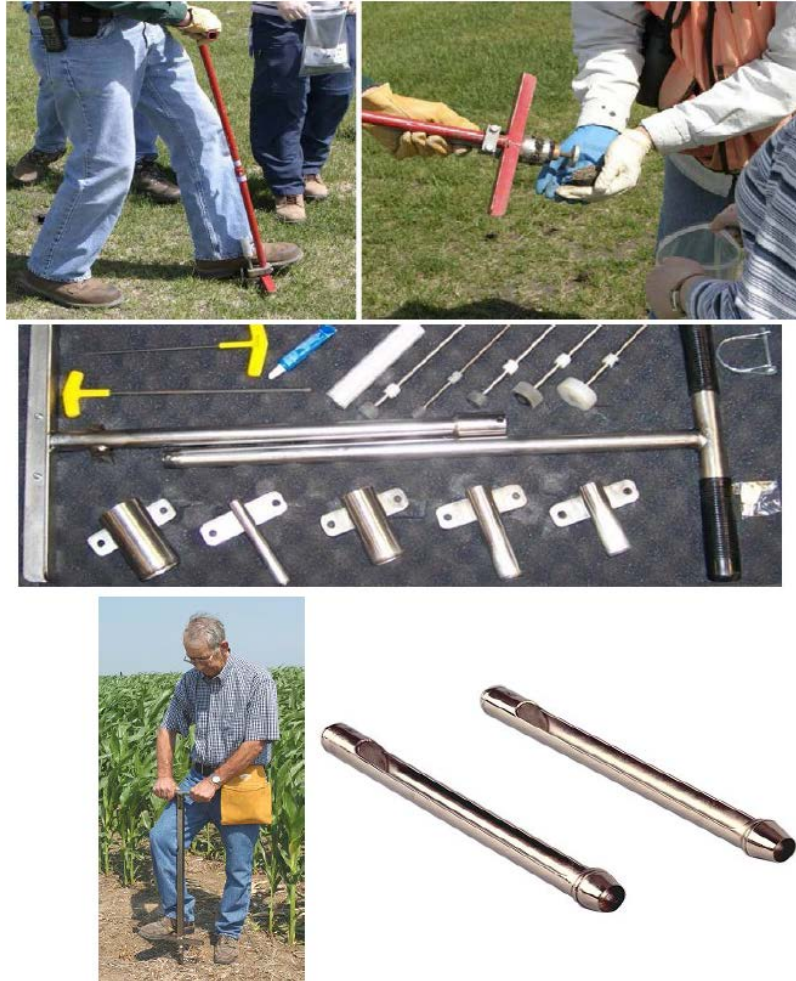
Figure 1: Examples of coring devices for non-volatile sample collection: Top to bottom: Multi-Incremental Sampling Tool (MIST™), EVC Incremental Sampler, JMC Backsaver Handle, and Soil Tube. (ITRC, 2012)
